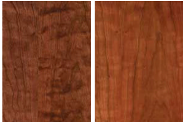
Finishing cherry requires extra attention, as these two panels from the same log show. The panel on the left was not pretreated with a wood sealer and has a blotchy appearance; only stain and a topcoat were applied. The panel on the right was treated with a sealer, followed by stain and a topcoat.
